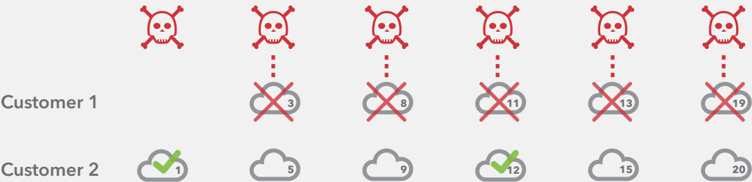
Figure 3: Akamai can manage name server delegations to further minimize the impact of an attack (compared with Figure 2, above), such as by moving a targeted customer off of an individual cloud and minimizing the overlap for nontargeted customers.
