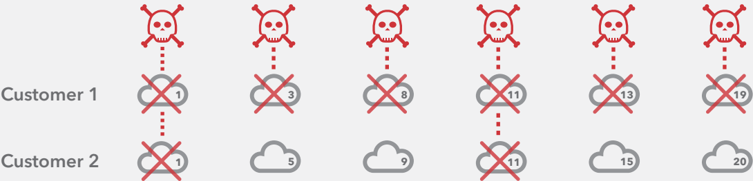
Figure 2: Every Edge DNS customer receives name servers on a unique combination of performance and availability clouds, minimizing the collateral damage from an attack against other customers.
