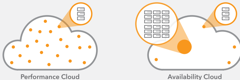
Figure 1: Edge DNS combines multiple DNS clouds with different architectures to offer an optimal combination of performance, availability, and resiliency against DDoS attacks.
