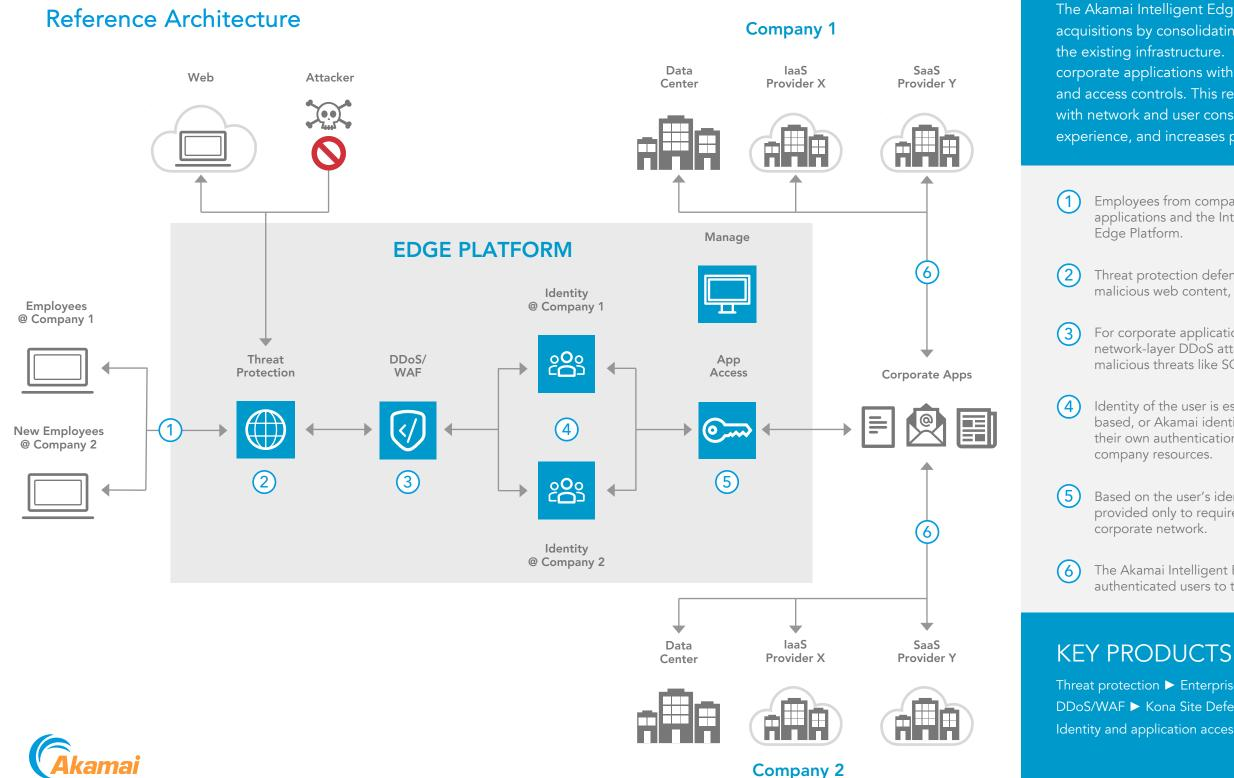
The Akamai Intelligent Edge Platform accelerates mergers and acquisitions by consolidating multiple networks without changing the existing infrastructure. It provides new employees access to corporate applications with the efficiency of a single set of security and access controls. This reduces complexity and cost associated with network and user consolidations, improves end-user experience, and increases productivity.
